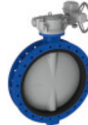
Series 820/20 Centric butterfly valve with loose liner U-section Ductile iron DN150-1600 With any type of actuation
