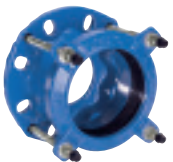
Series 603 Supa® flange adaptor Universal for cast iron, ductile iron, steel, uPVC and asbestos cement pipes Ductile iron DN40-400
