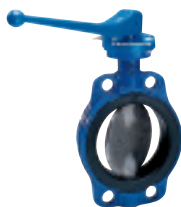
Series 75/31 Centric butterfly valve with fixed liner Semi-lug Ductile iron DN50-300 With any type of actuation
